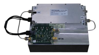
Figure 1:50W Class AB 2.45GHz amplifier with external ALC board
