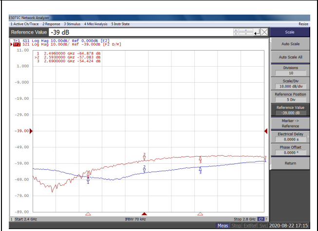
REVERSE OBSERVATION PATH TXIN TO OBS OUT (OUTPUT LOADED)
