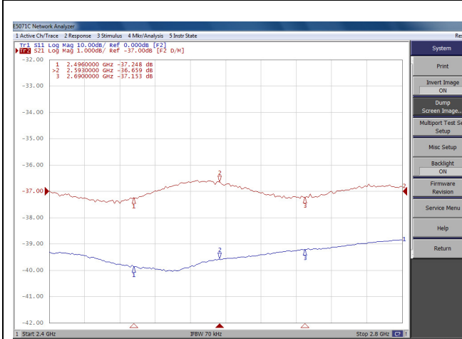
REVERSE OBSERVATION PATH TXIN TO OBS OUT (OUTPUT OPEN)
