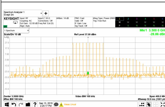
10 tones, 3500MHz, instant band = 76MHz, 5Wave, 28V/0.85A
