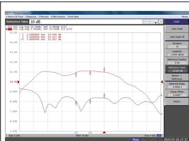
GAIN RX LINE UP WITH BYPASS
