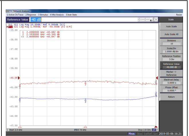
OBSERVATION PATH RELATIVE TO TX OUTPUT
